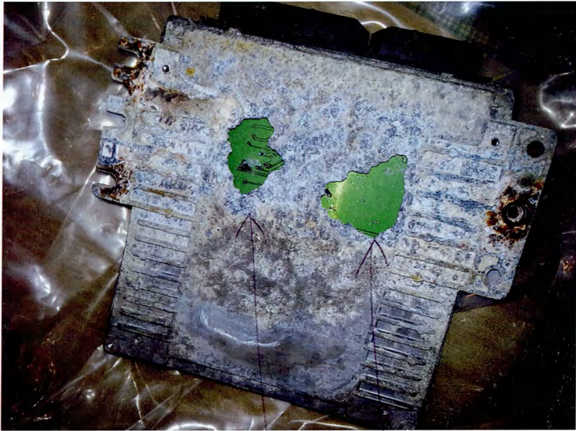
Figure 1: Corroded ECM from my 2004 Nissan Quest due to the faulty design
