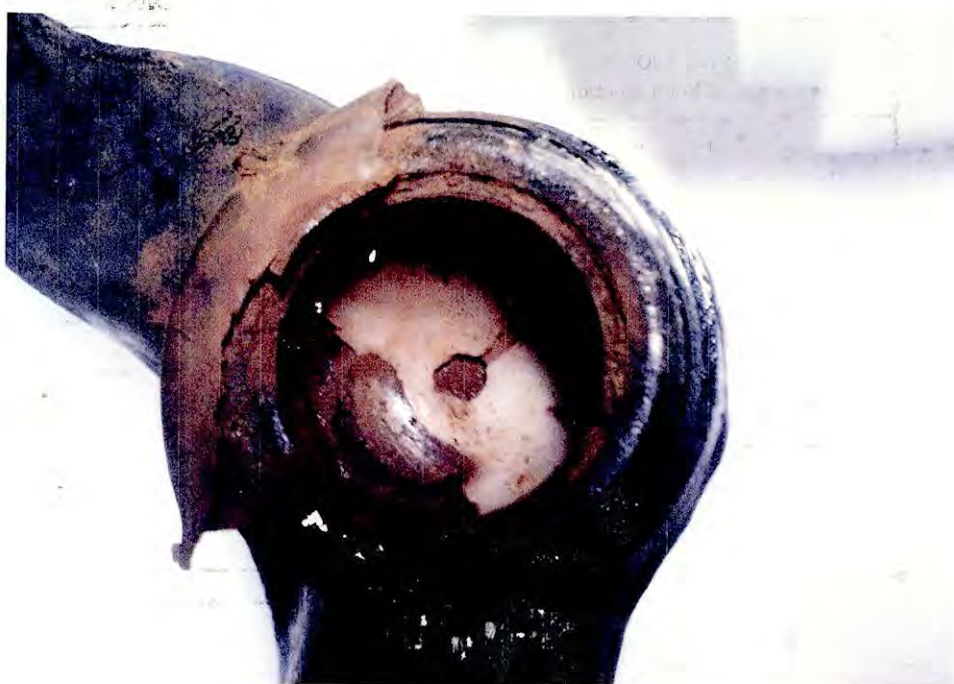
Rusted Ball Joint Socket
