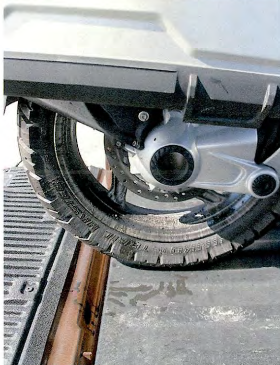
Rear tire and brake after the final drive bearing failed
