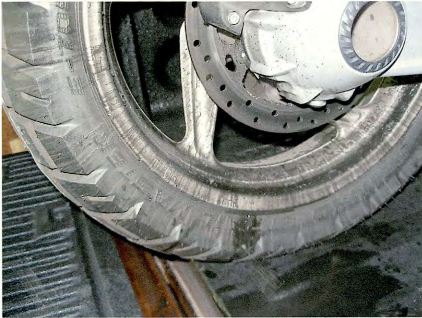
Rear tire and brake after the final drive bearing failed
