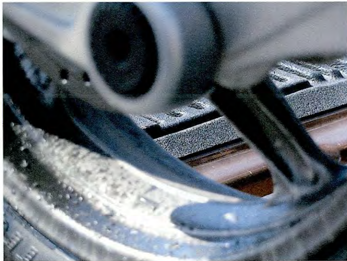
Rear tire and brake after the final drive bearing failed
