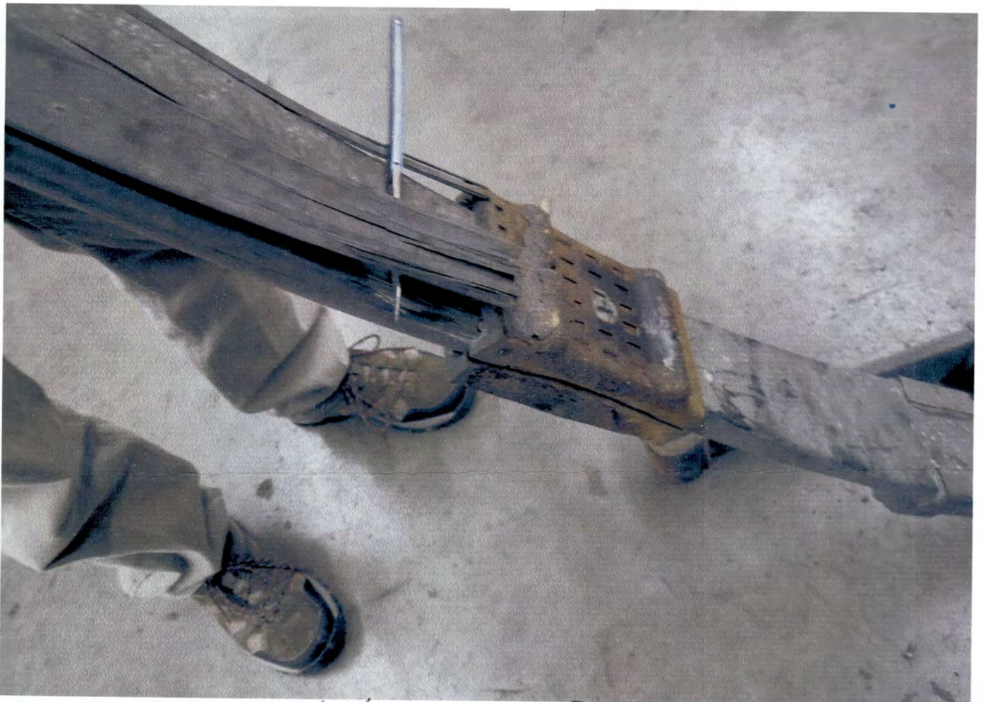
Shows splintering of Spring near AXLE SUPPORT
