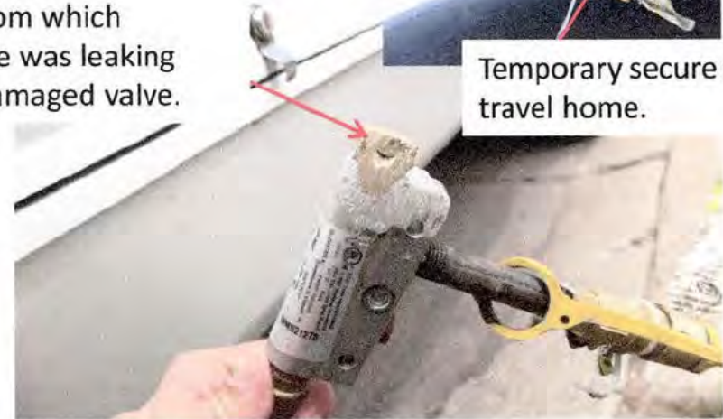
Additional damage to valve assembly.
