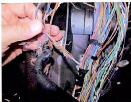
Notes: BLACK WRAPPING AT BOTTOM TO SEAT- -NOTE KINK IN COVER AND THEN BURNE, MELTED WIRING-RED/BUE WIRE APPEARS TO HAVE SOME CORROSION Esc -Exit Page Down/Up - Next/Previous Image
