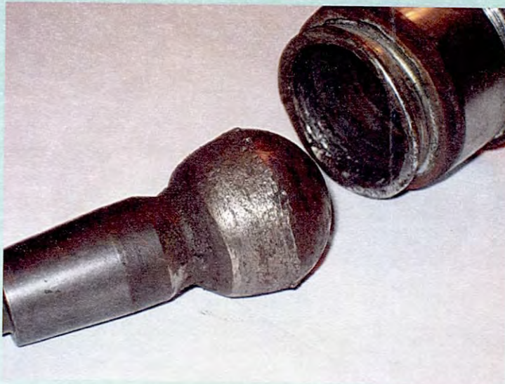
Removed Ball joint showing failure
