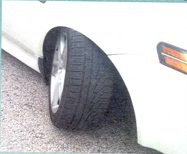
Front wheel after ball joint failure
