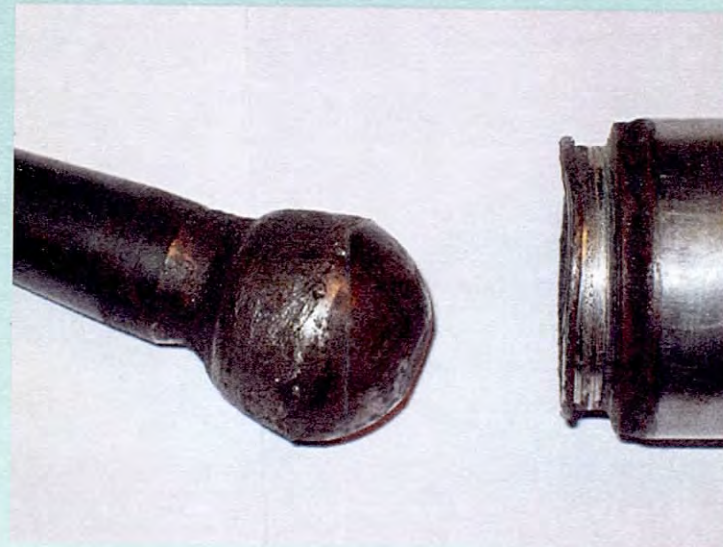
Removed Ball joint showing failure
