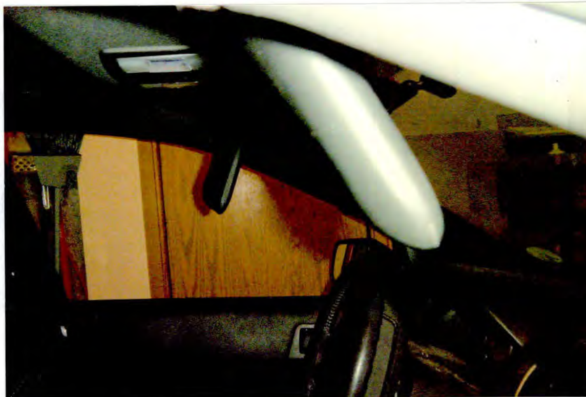
The driver's side visor is set in the 1 st position away from the "home" position. The passenger side visor is set in its 3rd position away from the "home" position.
