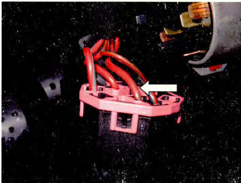
Photo of Mk4 Golf Ignition Switch Connector at Tomas Sport Tuning in Berkeley, CA
