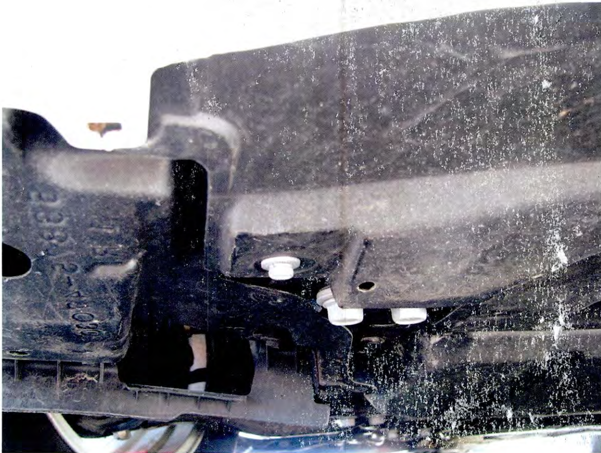
Close shot of plastic undercarriage shielding located at right front wheel (viewed from front of vehicle). Note no presence of scratching to indicate under-carriage collision.
