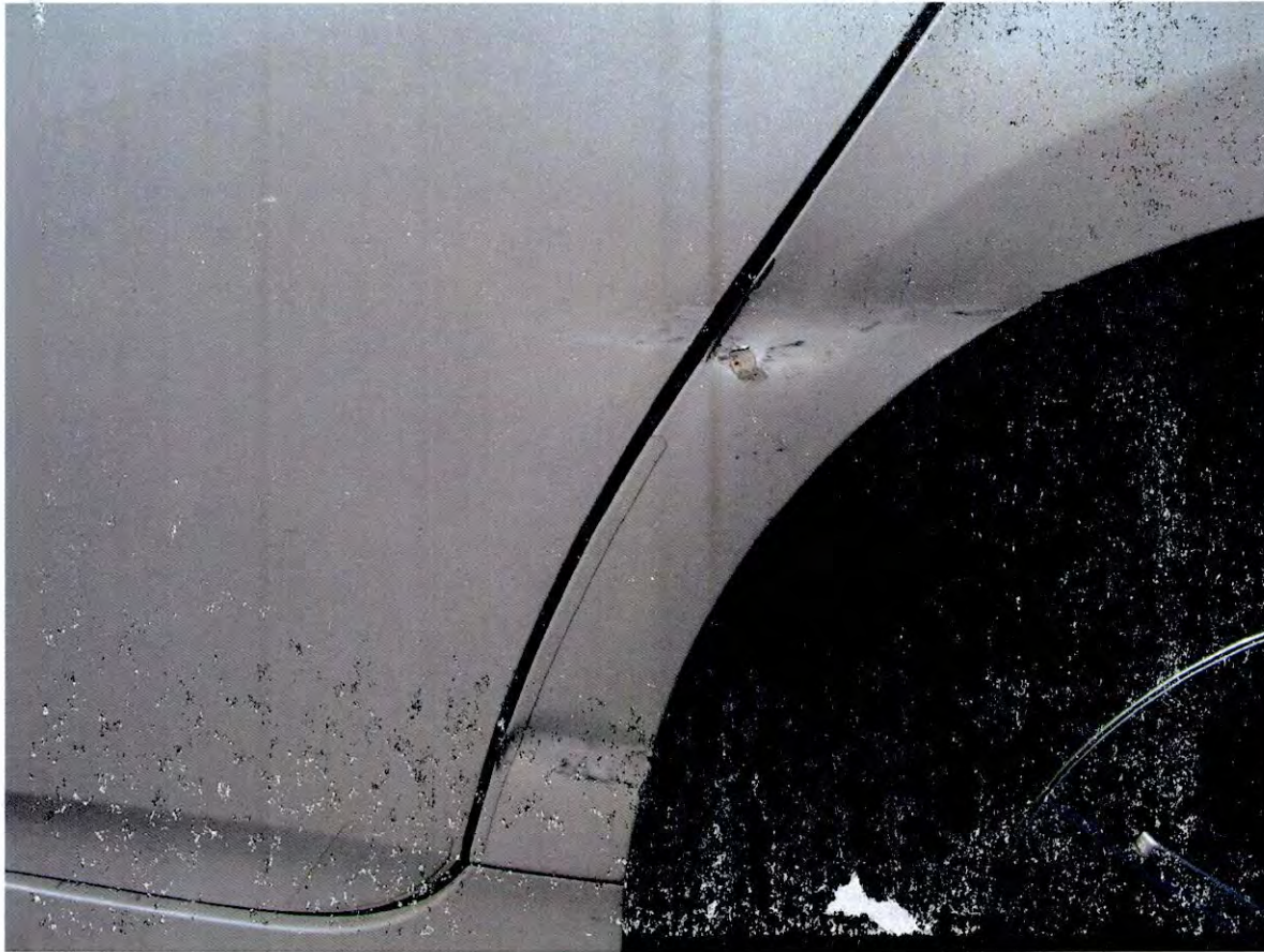
Close image of rear quarter panel showing slight dent and scratching from light contact with galvanized highway guardrail.
