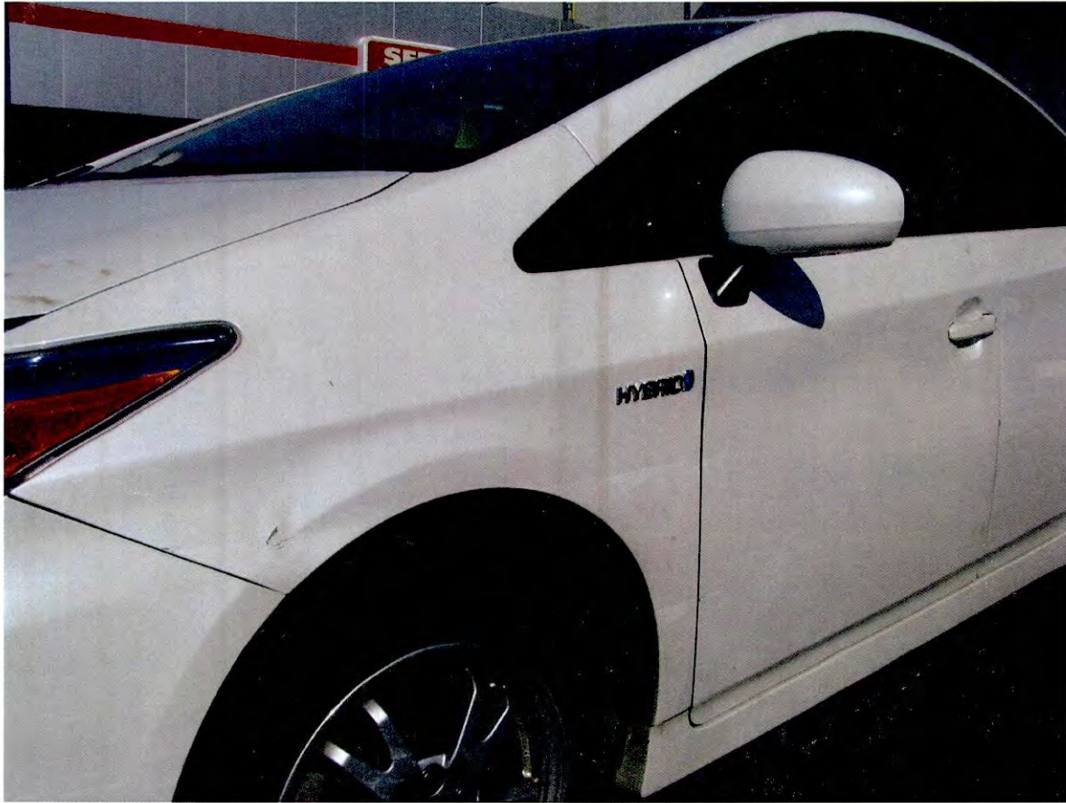
Driver side of vehicle showing light scratches and denting on front quarter panel from light contact with galvanized highway guardrail. Note 0 degree (straight) orientation of left front wheel.
