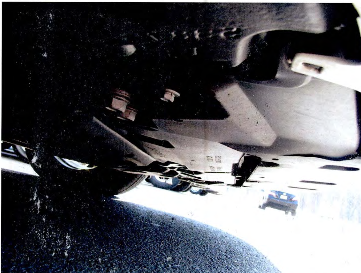
Underpanel of vehicle as seen from right front corner of vehicle. No presence of scratching to indicate under-carriage collision.
