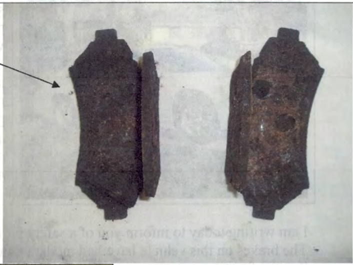
Front outer pads. Still serviceable but replaced due to premature failure of inner pads
