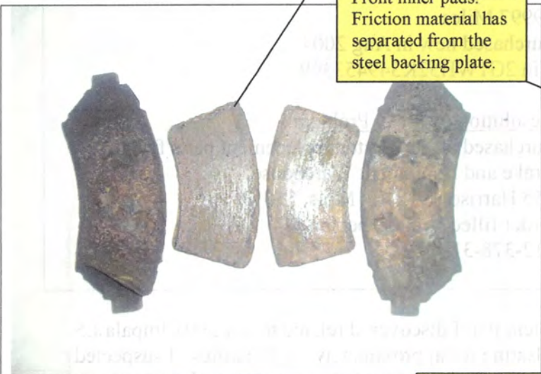
Front outer pads. Still serviceable but replaced due to premature failure of inner pads
