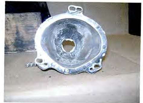
Illustration F. Showing degraded surface inside reflector causing loss of illumination ahead of vehicle.
