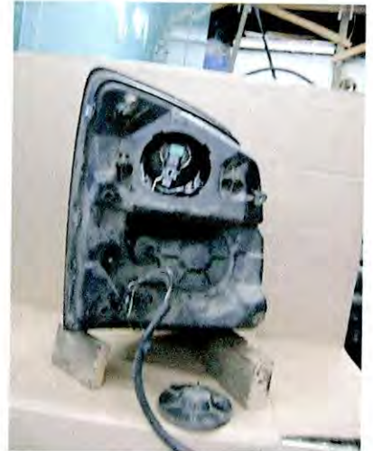
Illustration C. Showing removed cover to replace bulb.
