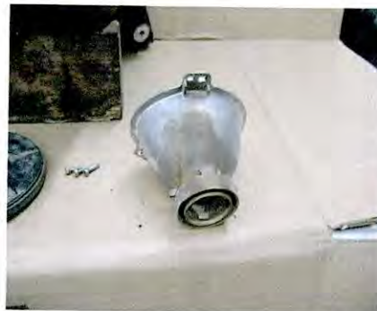
Illustration E. Showing reflector removed by taking out 3 screws. Notice burned surface on top.
