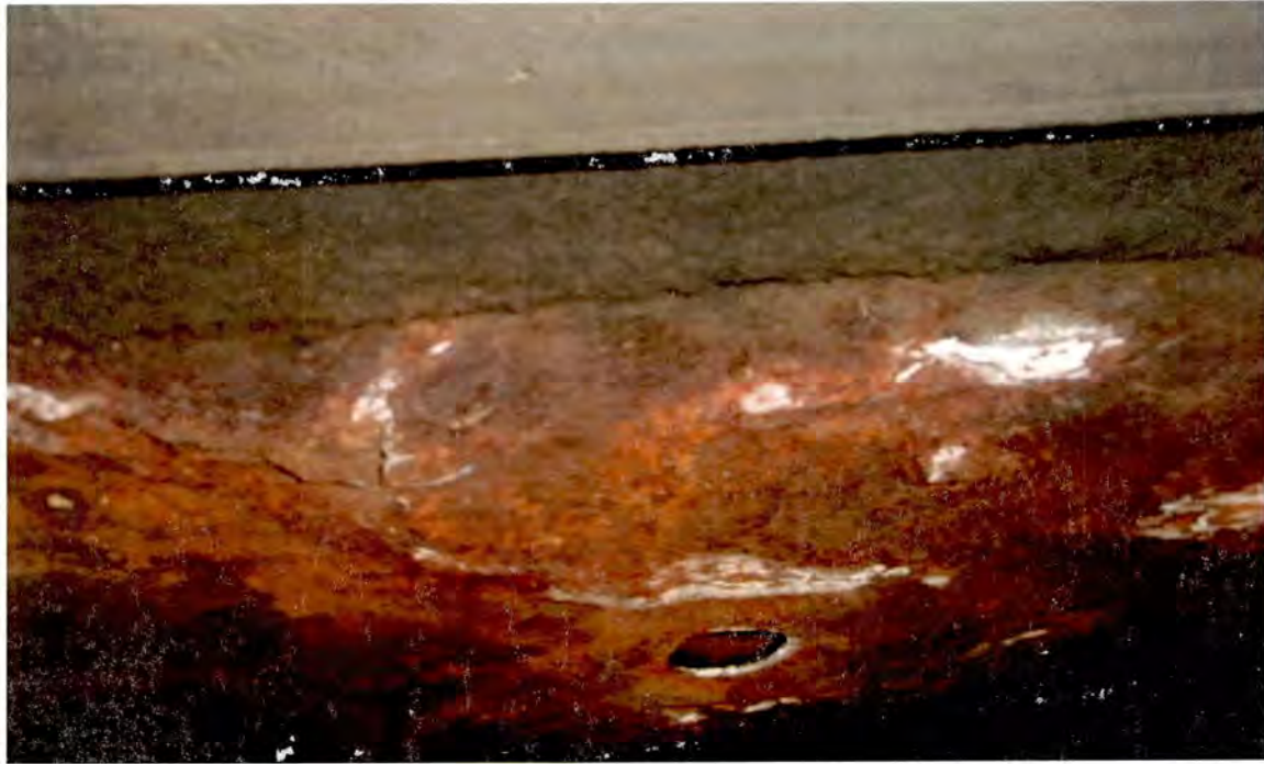
Break in steel plate due to corrosion surrounding manufactured hole in plate, MN license plate # [REDACTED]
