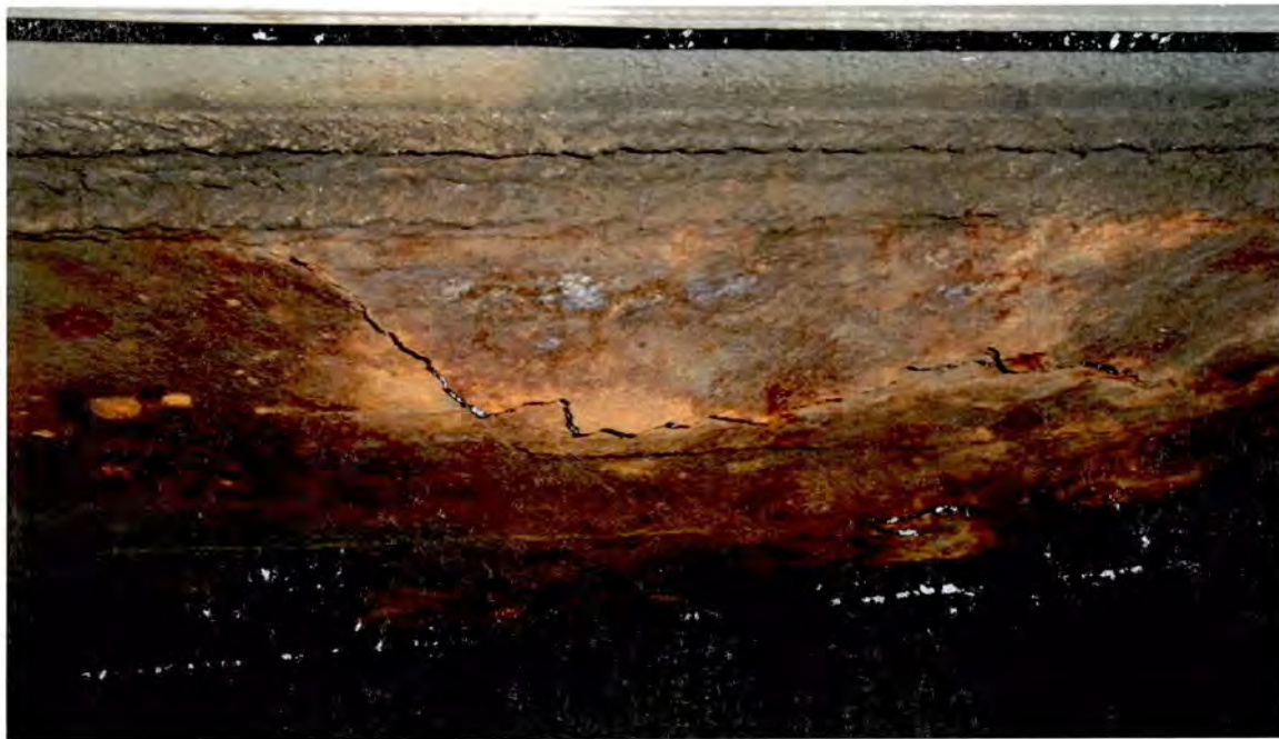
Break in steel plate due to corrosion surrounding manufactured hole in plate, MN license plate # [REDACTED]
