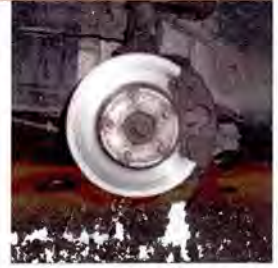
Damaged brake rotor from metal-to-metal contact
