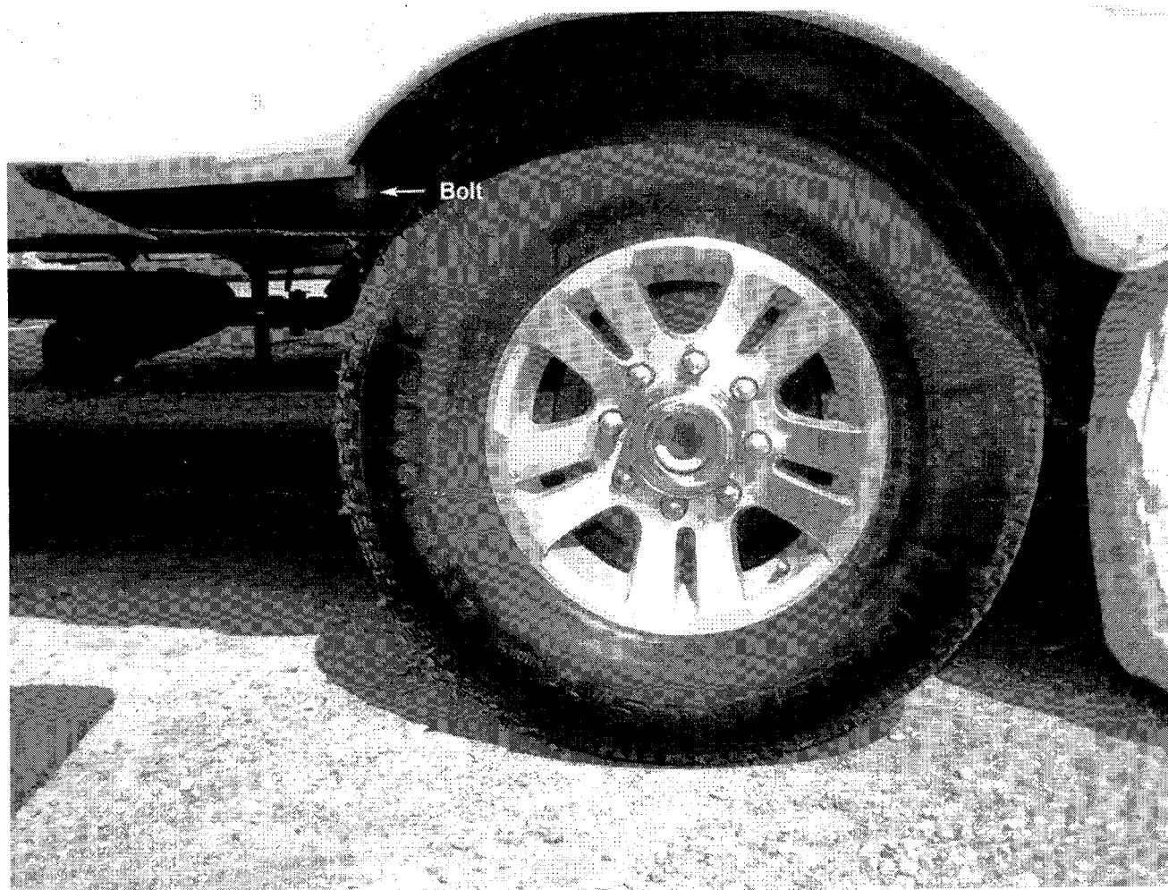
Photo of bolt that cut the tire after the hanger on leaf-spring broke
