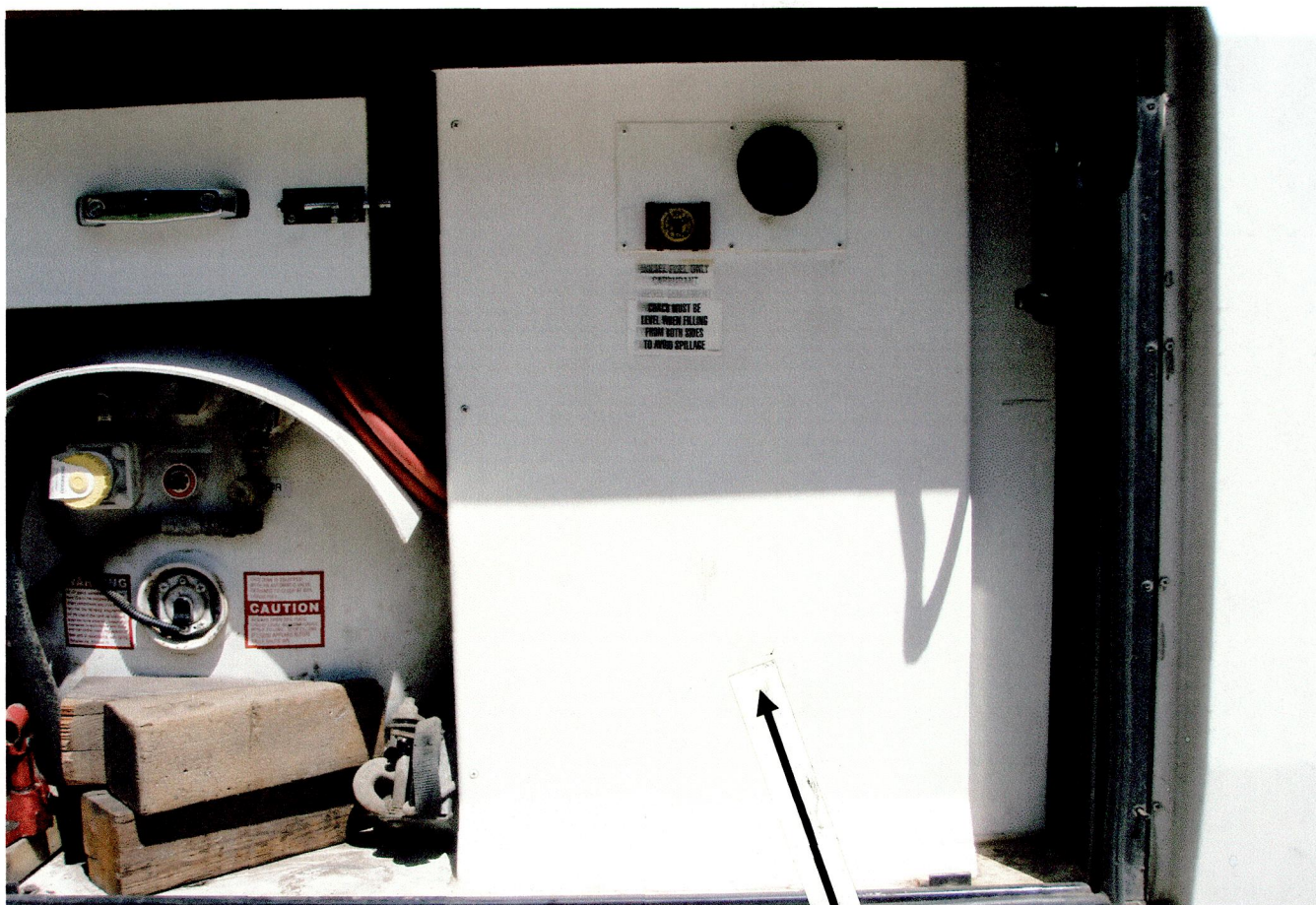
PICTURE 1 FOREWORD PASSENGER SIDE BAGGAGE COMPARTMENT W/ FIBERGLASS COVERING OVER ALUMINUM FUEL TANK
