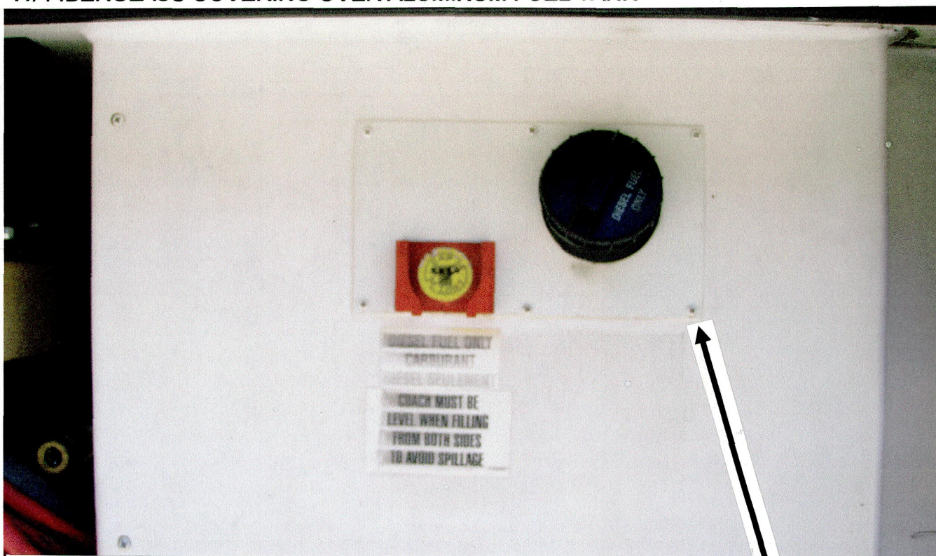
PICTURE 2 FIBERGLASS COVERED ALUMINUM FUEL TANK. CLOSE-UP VIEW OF 4.5" X 8" SECONDARY FIBERGLASS COVER SURROUNDING FUEL FILLER NECK. NOTE: 6 SCREWS SECURING SECONDARY COVER.
