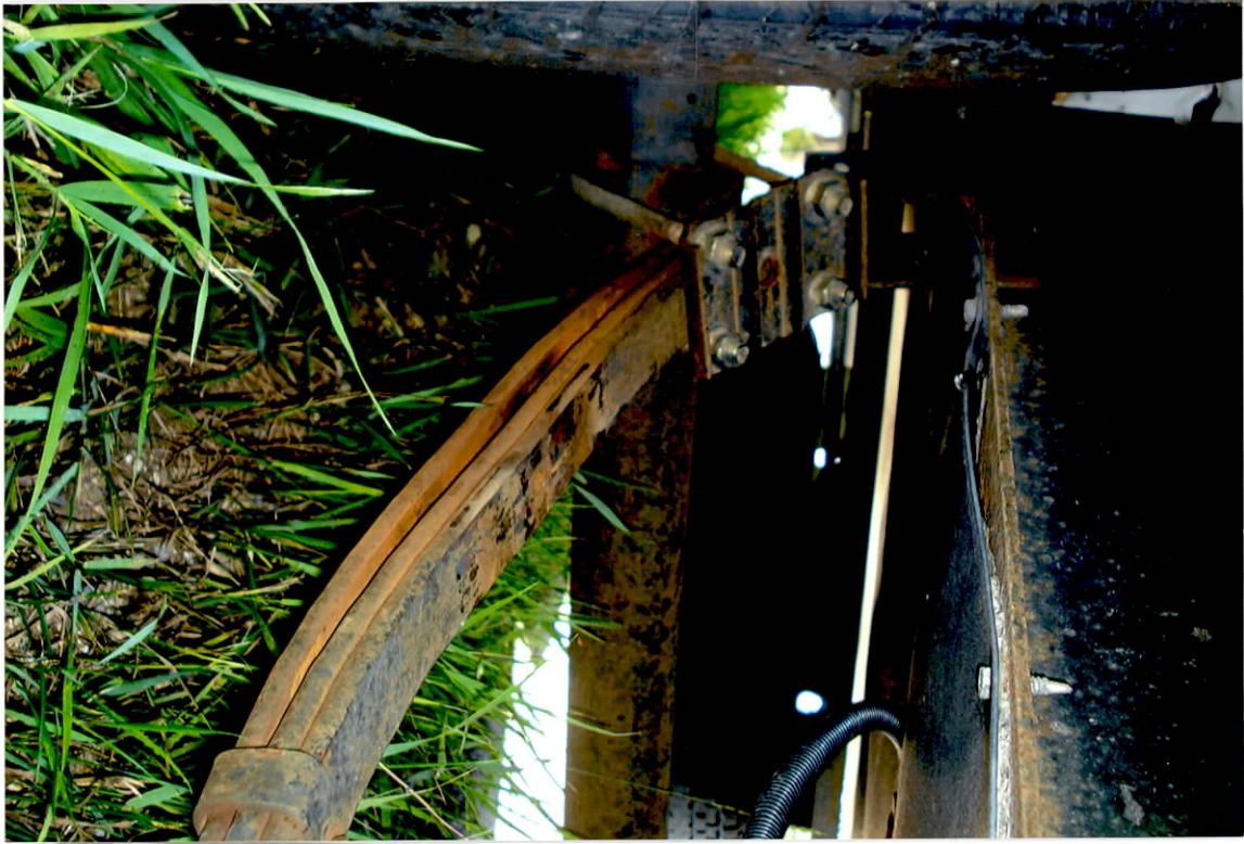
Axle resting on hanger after sliding back and Shows 2 shorter leaf springs as they were gone & laying on road
