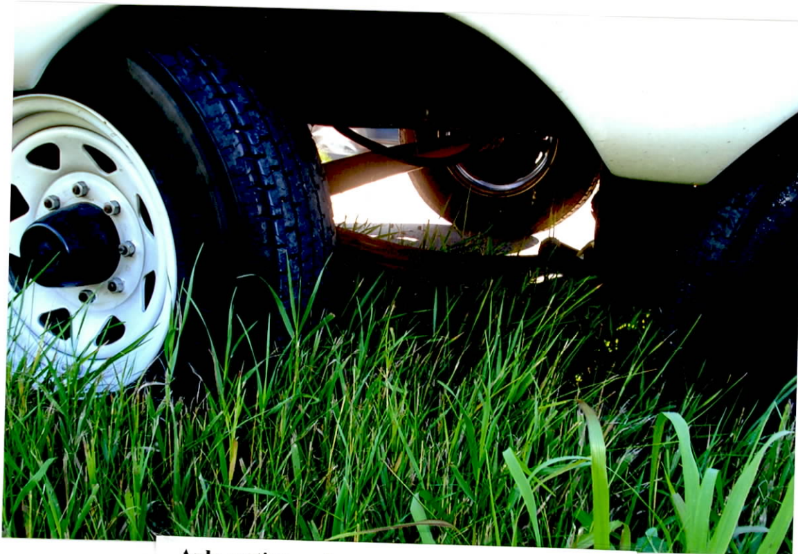
Axle resting on hanger after sliding back
