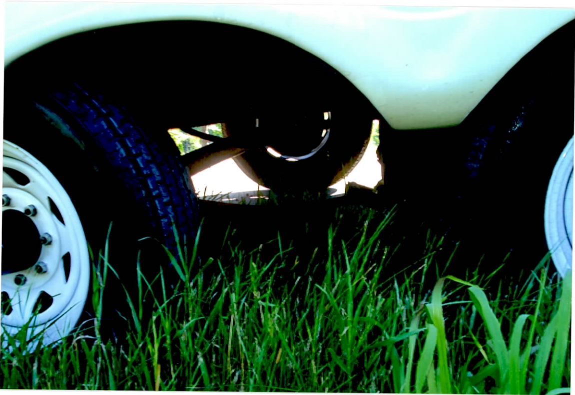
Distant picture of axle slid back on spring shackle
