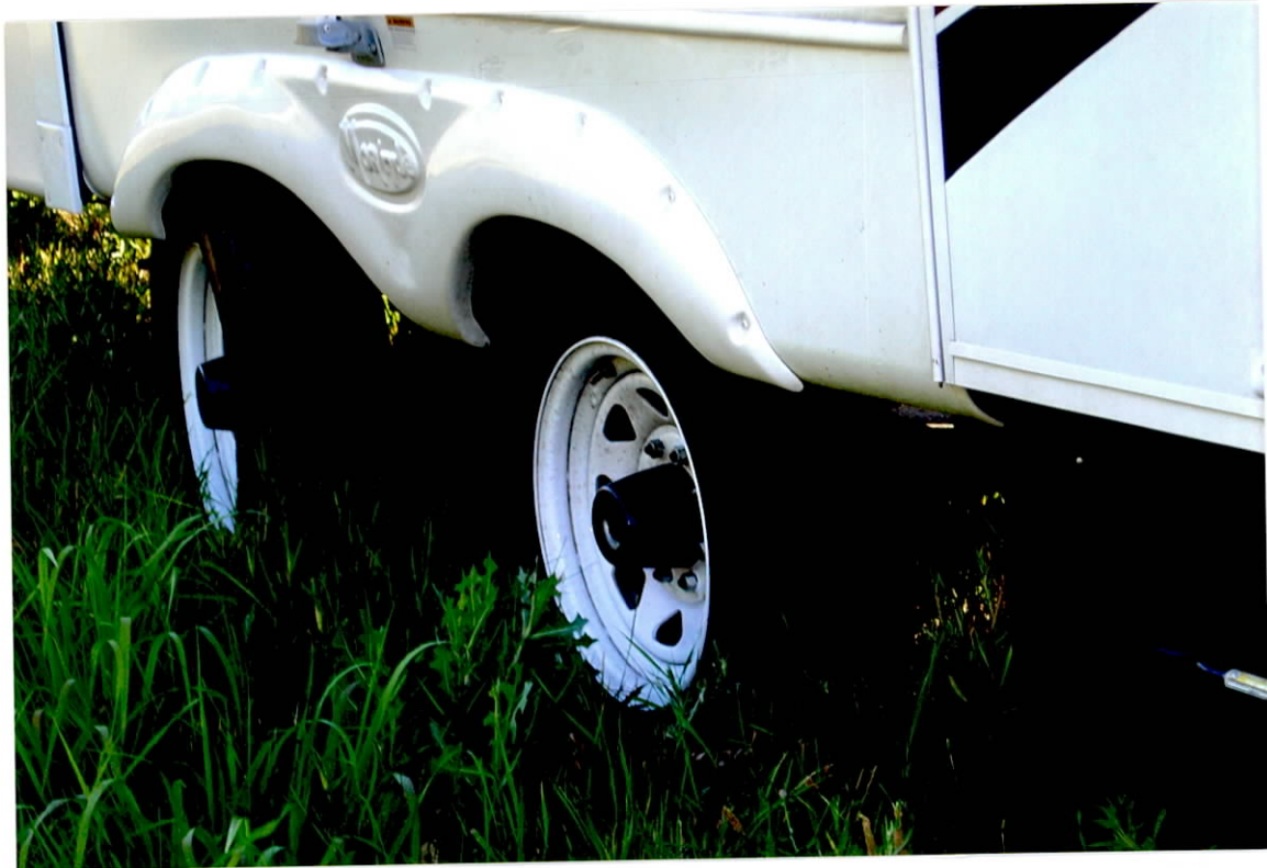
Another angle showing view of axle slid back under camper
