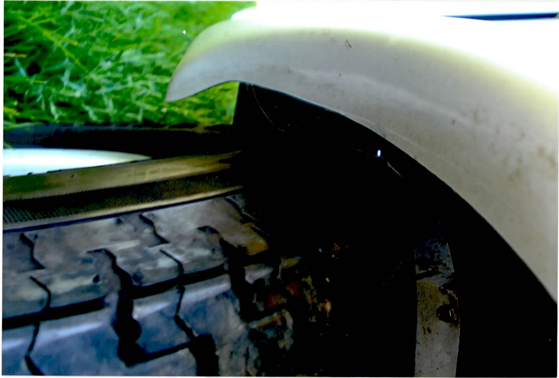
Axle resting on hanger after sliding back and Shows 2 shorter leaf springs as they were gone & laying on road
