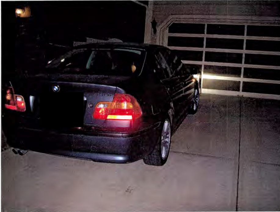
Photo 1 – Rear View of Tail Lights with Head Lamps on and 4 Way Flashers Operating. Only the lights in the trunk lid are operational
