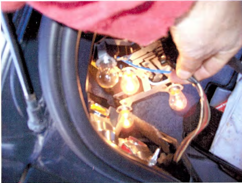
Photo 3 – Tail Light working with pressure applied to tail light / wiring harness connection. When pressure was removed tail light would malfunction.
