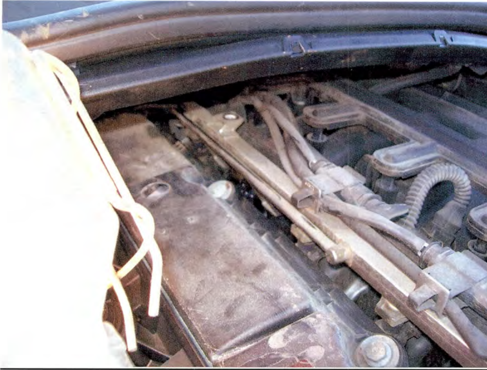
Photograph 1 – It is difficult to see with the lighting I had, but there is quite noticeable dampness/darkness due to gasoline leak around fuel injector no. 5.
