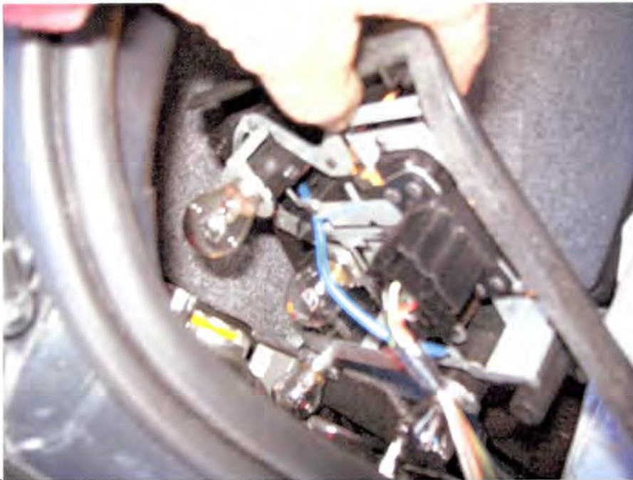
Photo 2 – LHS Rear Tail Light Assembly , tail lights a 4 Ways on, connected but not working.
