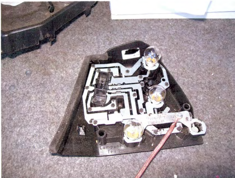
Photo 4 – This shows the modification made to the tail light assemblies to improve the grounding of the tail light assembly.
