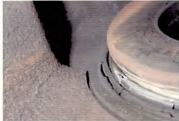
A cracked piston dust seal/boot can be a warning sign.
