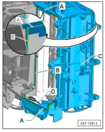
Insert the grooves <A> on the right heater core housing into the guides on the A/C unit <B> and push the right heater core housing <C> just a little into the A/C unit.
