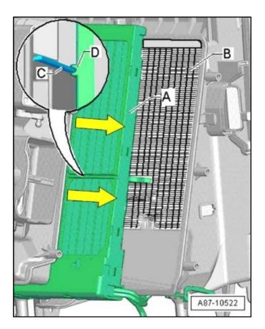
Remove the Auxiliary Heater Heating Element -Z35- <A> from the A/C unit in direction of <arrows>.
