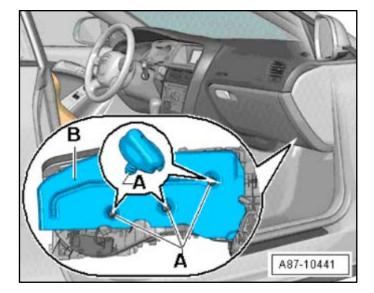
Install insulation mat <B> and tighten screw clips finger tight.
