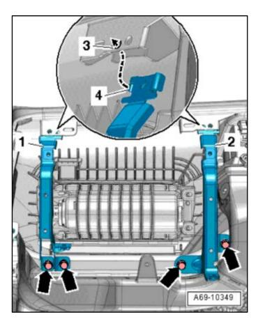
Remove bolts <arrows> and remove glove compartment mounts <1 and 2>.
