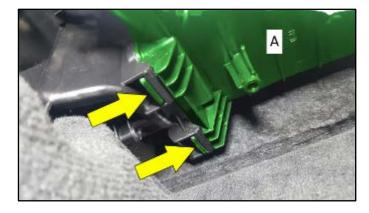
Remove air intake housing <A> off the mounts <arrows> and remove air intake housing from the vehicle.
