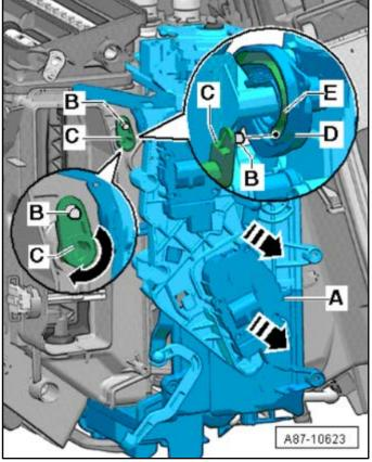
Pull the right heater core housing <A> (together with the retaining plate, actuators and levers, curved washers and connecting rods) in the direction of the <arrow> from the A/C unit.
