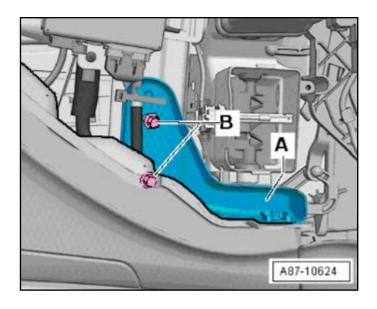
Remove the two bolts <B> and remove the bracket <A>.
