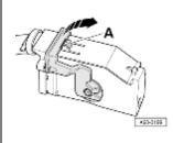
To disconnect the connector, press the tab <A>, turn the retaining bracket in direction of <arrow> and remove the connector.
