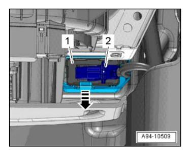
If equipped, install the Headlamp Range Control Module <1> and connect connector <2>.
