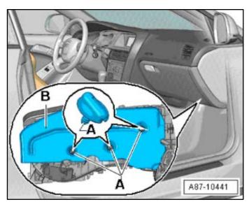
• Remove the screw clips <A> and remove the insulation mat <B>.
